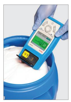
The analyzer performs identification through sealed packaging to minimize the risk of contamination and exposure.
